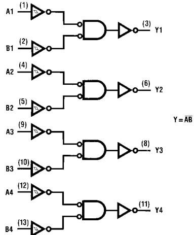
MM74HC132 Quad 2-Input NAND Schmitt Trigger
