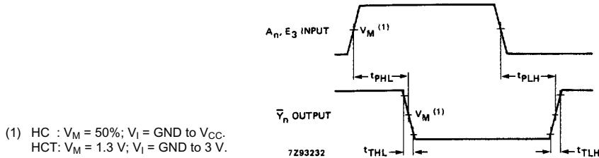
Fig.6 Waveforms showing the address input ( $A_n$ ) and enable input ( $E_3$ ) to output ( $\bar{Y}_n$ ) propagation delays and the output transition times.
