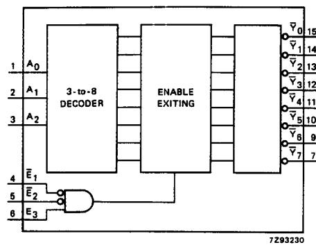
Fig.4 Functional diagram.
