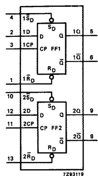
Fig.4 Functional diagram.
