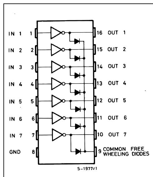
**ULN2001A - ULN2002A - ULN2003A - ULN2004A****SCHEMATIC DIAGRAM**
