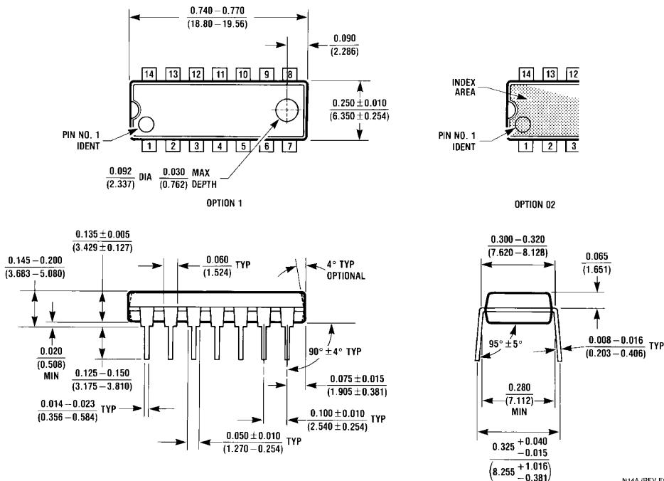
14-Lead Plastic Dual-In-Line Package (PDIP), JEDEC MS-001, 0.300" Wide
