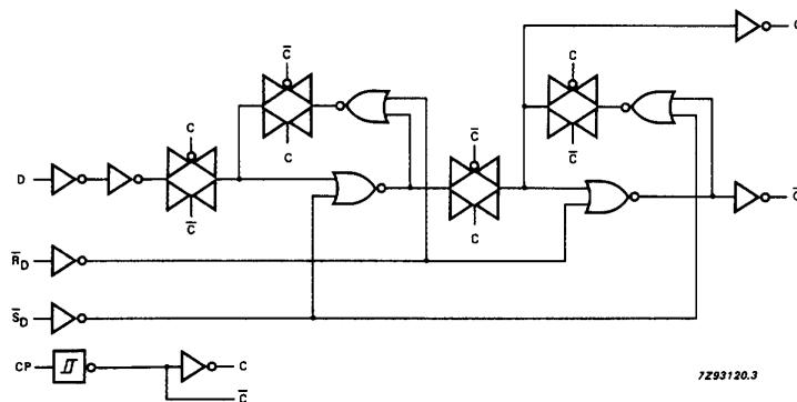
Fig.5 Logic diagram (one flip-flop).
